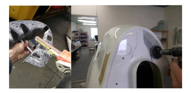
After cleaning these surface, apply epoxy on them for a better bounding of the glue and continue before drying out of this epoxy
