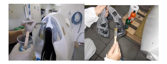
Add to approximately 50g of epoxy the white fibre mix added to the kit. Mix well till you have a uniform pasta. If it is still flowing, add some more fibre mix. Introduce this in a plastic bag and cut one angle out so that you can apply the glue on the carbon part there where it will touch the body.
