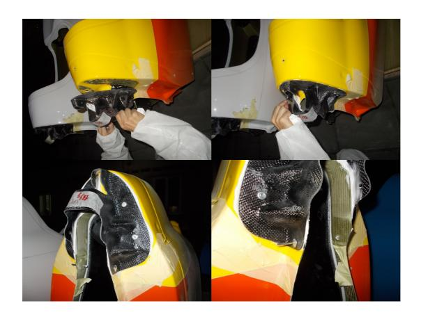
The body of model WAW@2014 has shorter lateral edges around the rear wheel and after gluing the carbon part, some openings between this part and the body need to be closed to prevent from entering water and dirt. This can be done by laminating 2 bands of fibres over them. Do not add material 15 mm around the axle of the upper swing during this operation.
