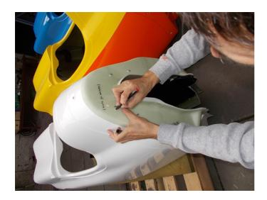
For an after-mount do not drill the highest hole (6mm  $\rightarrow$  20mm) on the jig. If the WAW has a connector for the lights in the tail, the existing hole in the body will be transferred on the carbon part delivered in the kit. If the WAW has no connector towards the tail, this hole is not needed at all.
