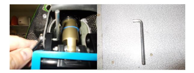
Now attach the upper part of the shock. Note the reduction tube from diameter 8 to 6mm in the shock. Tighten well enough the safety nut so that the shock moves around the aluminium bushings.
