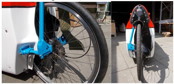
Braking on the rear wheel of a tadpole trike can be hazardous but some mountain countries ask for the possibility of additional braking capacity. Therefore, the left drop-out has been standardly adapted to mount a disc brake for 180mm discs.
