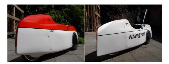
Tail T1 is much shorter and if you wish to fit the rear suspension the cut-out for the wheel will end higher and it will be necessary to use a thin tire of maximal 35mm.
