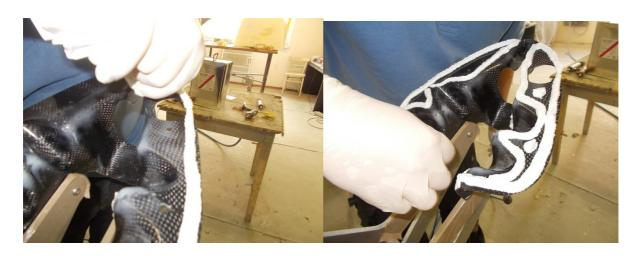
Put the carbon part in place and introduce the rivets. Rivet them all except the one at the left under, directing towards the rear wheel well, which will only be riveted after the glue has hardened. Remove all excess glue and clean with alcohol. Let harden for 24h.
