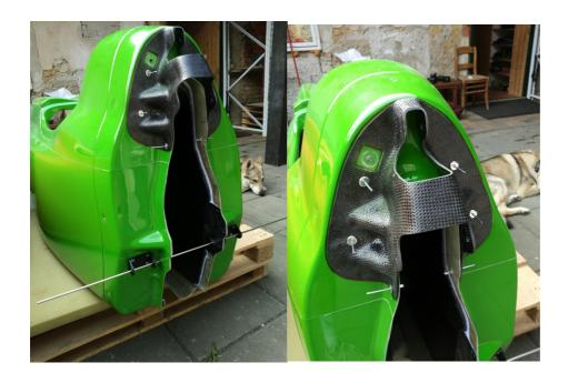
If the WAW has a connector for lights in the tail, you must at this moment copy the hole of the connector in the body to the new carbon part, as well as the holes for the screws. Afterwards you cut this out in the carbon part in such way that the head of the screws rest directly on the body so that the connector coming from the tail can enter deep enough on the connector on the body.
