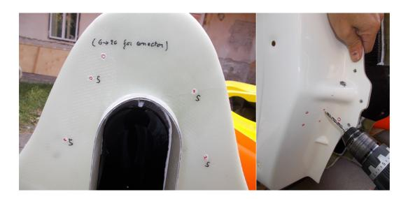
Test the position of the carbon part by putting it in place and pushing the rivet manually in the holes. If needed, drill again through the holes which are not on top of each other without moving too much the carbon part. The axle of the lower swings must be in line with each other. If necessary make the hole with 8mm diameter a little bigger so that the M6 screws, axles for the lower swings, can be mounted well.
